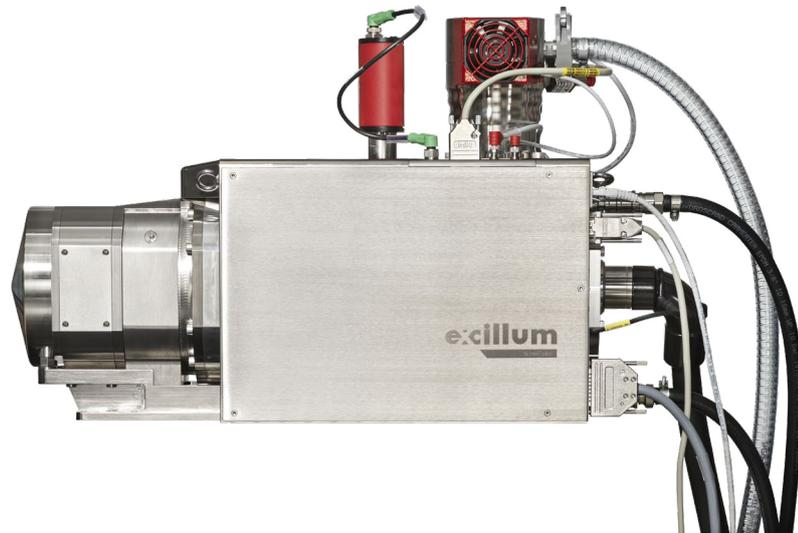
The Excillum NanoTube N3 enables industry-leading resolution and stability in geometric-magnification X-ray imaging systems with no need for manual tuning. It is based on advanced electron optics and the latest tungsten-diamond transmission target technology. Automatic e-beam focusing and astigmatism correction ensures that the smallest possible, truly round spot is achieved every time, every day.
